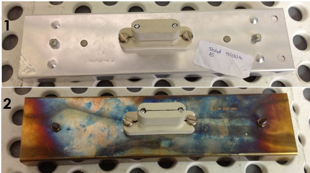
Figure 2: Comparison of aluminised steel (1) and stainless steel (2) after testing.
